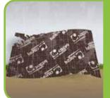
After the formwork is dismantled, inspect the plywood. Remove any excess concrete. Do not use severely deformed sheets for further works. If damage is minor, use the sheets for non-standard elements
